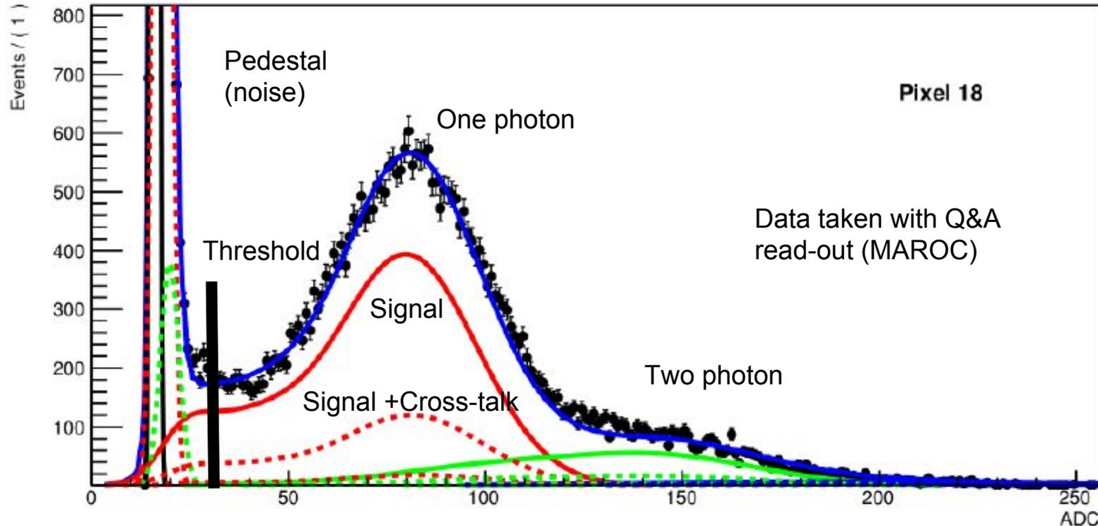
The MaPMTQ&A model was developed for PMT Q&A will be used to fit the threshold scan
