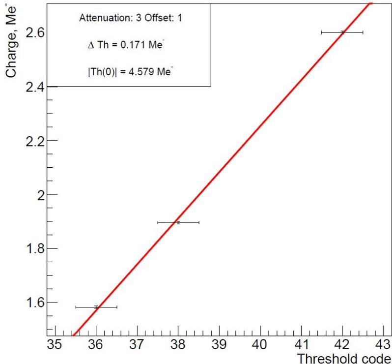
**Step 1:** for a given threshold value known amount of charge is injected to CLARO (DAC scan)
