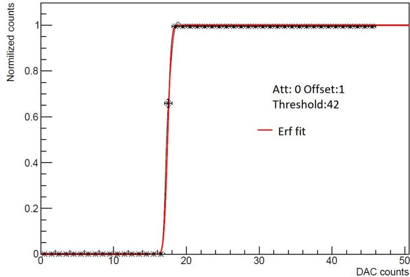
**Step 1:** for a given threshold value known amount of charge is injected to CLARO (DAC scan)
