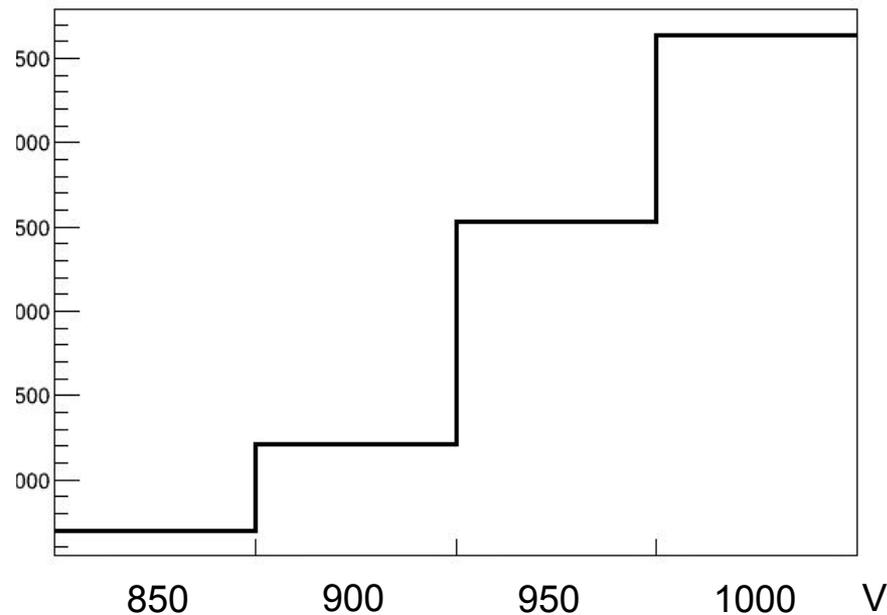
Mean gain for TT A channels at different voltages
