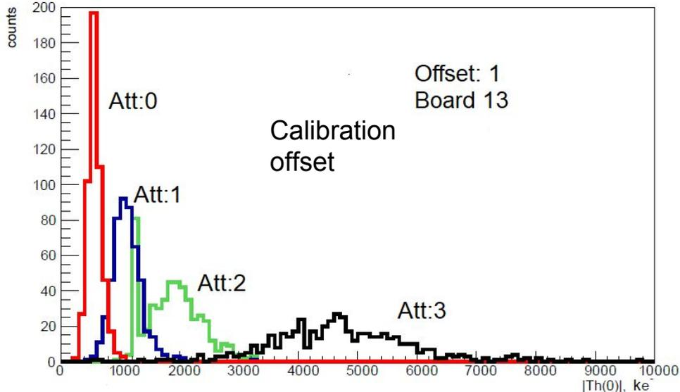
Attenuation: attenuation of signal in  $2^{att}$  times.
