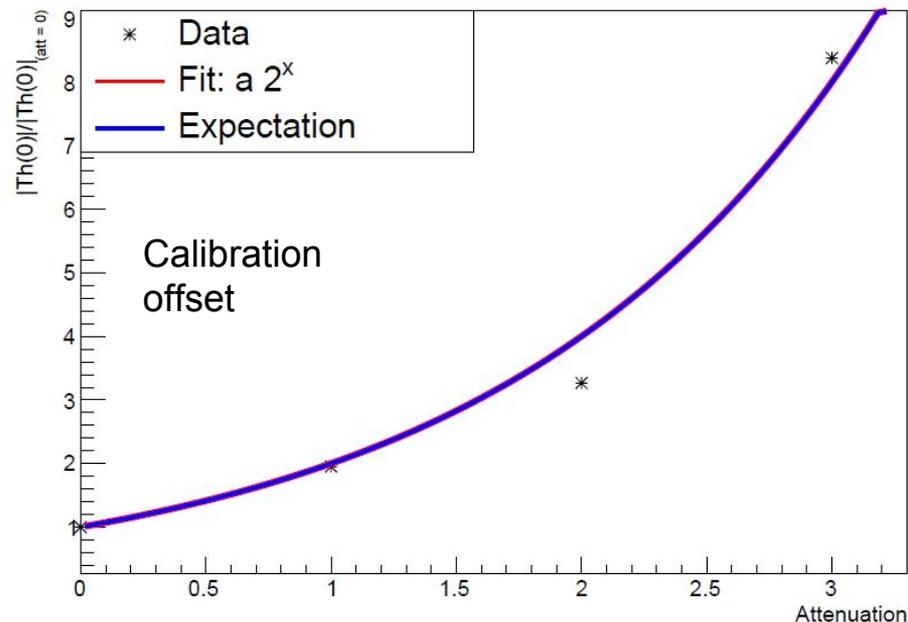
Averaged over all channels results on  $\Delta Th$  and  $|Th(0)|$  for different attenuation
