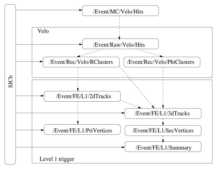
the dashed lines represent the virtual dataflow as exists in SICb - the algorithms to make e.g. tracks from clusters are the next stage
