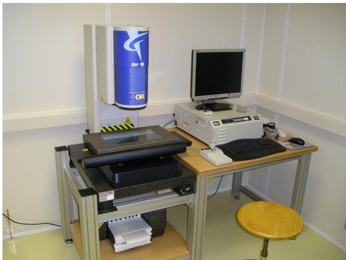
Optical 3D coordinate measurement machine (CMM) in PH/DT bond lab.
