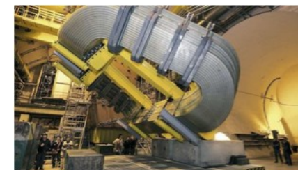
LHC-beauty, or LHCb, is an enormous detector designed to examine CP violation
