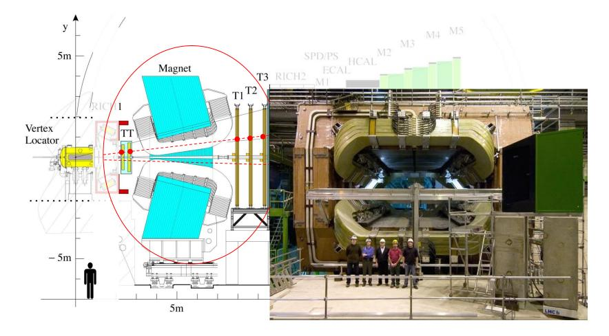
**Tracking system** and dipole magnet to measure angles and momenta  $\Delta p/p \sim 0.5$  %, mass resolution, together with VELO ~ 25 MeV (for B<sub>s</sub>  $\rightarrow \mu\mu$ )
