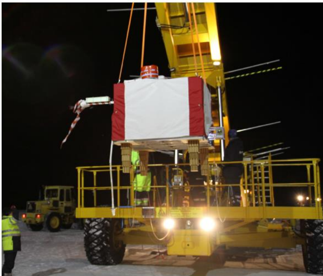
(a) The launch vehicle carrying the gondola with the experiments before the BEXUS-11 launch
