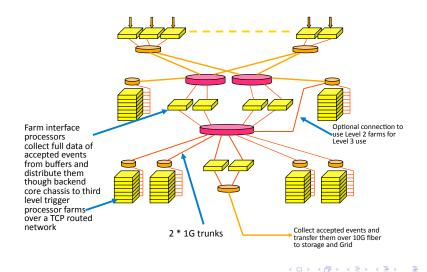
Efficiency Networking at the host side DAQ networks
