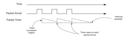
Figure: Receive packet timer to ensure timely delivery from ref. [10]
