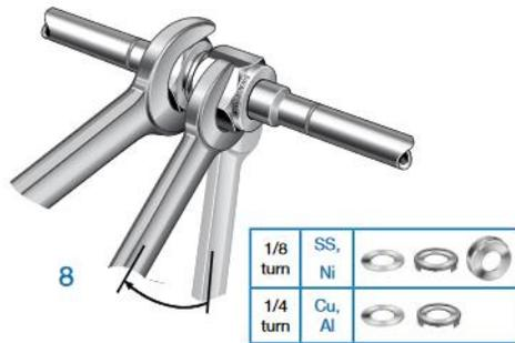
By connecting the VCR a torque on its pipes is introduced. This is due to the metal/metal seal
