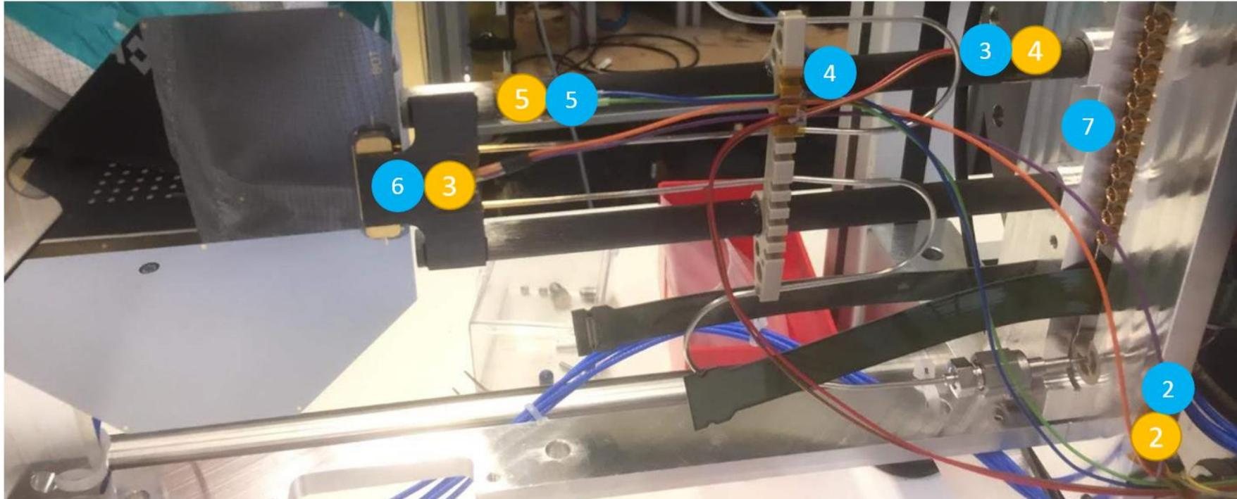
Numbers in blue are the PT100s that are on slide 26, In orange are the positions of the previous module.
