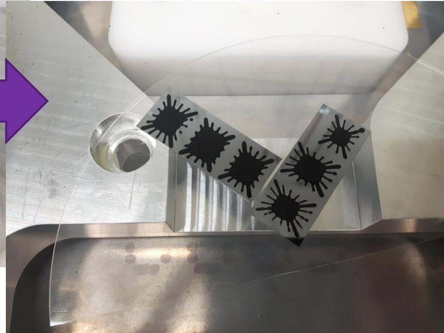
Glued to a glass plate, to check for spread.
