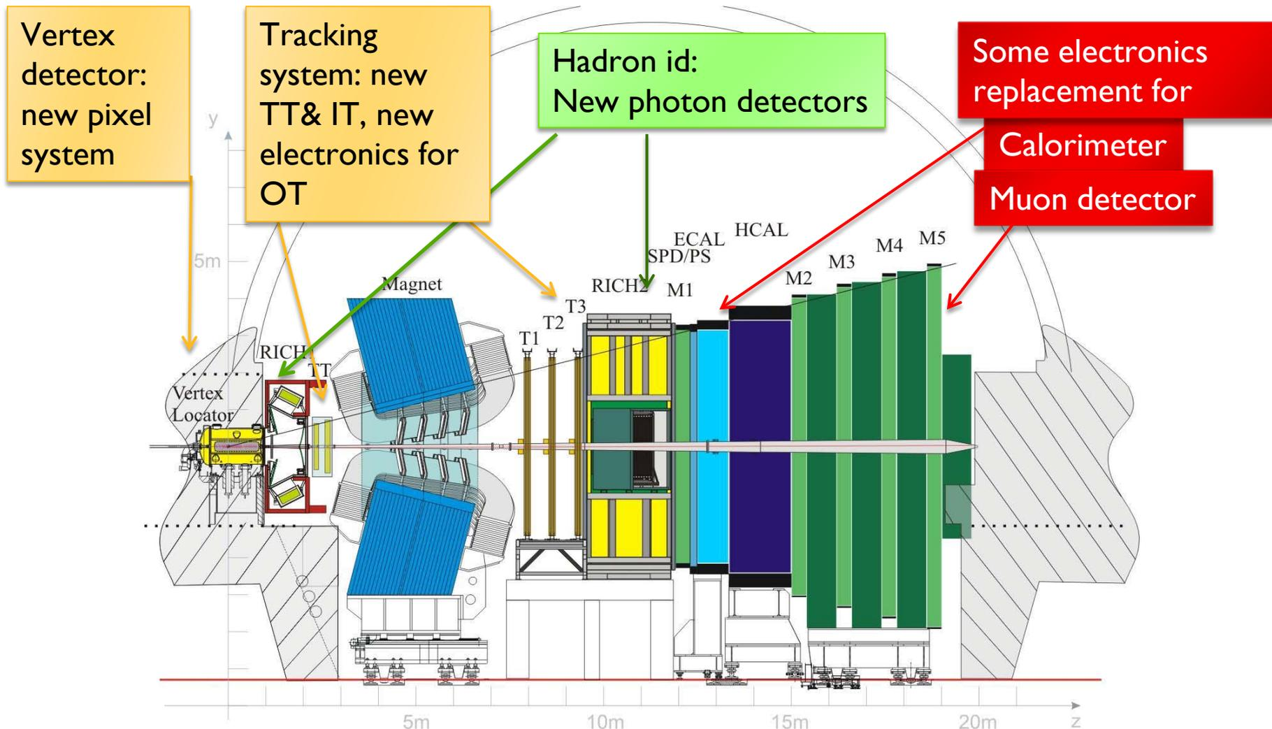
◆ Replace all the front-end electronics + DAQ network
