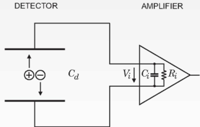
**SNR is inversely proportional to total capacitance on the input → thicker sensor gives more signal but also more noise**
