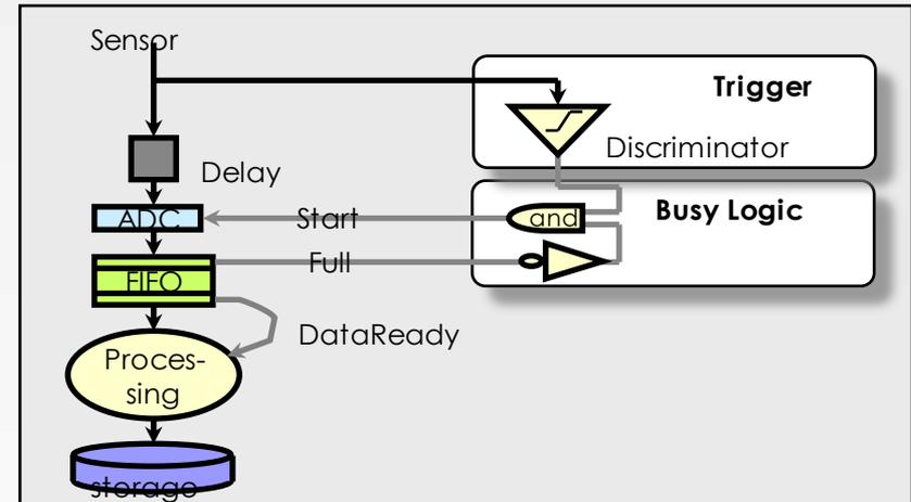
The system is *busy* during the ADC conversion time if the FIFO is not full (assuming the storage can always follow!)
