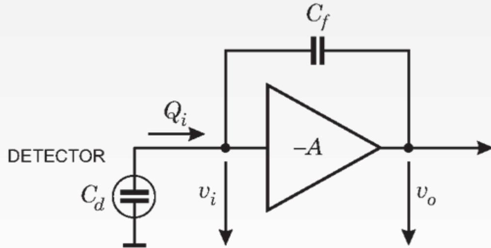
$$A_Q = \frac{v_o}{Q_i} = \frac{Av_i}{C_f(A+1)v_i} = \frac{A}{A+1} \frac{1}{C_f} \approx \frac{1}{C_f} \quad (A \gg 1)$$
