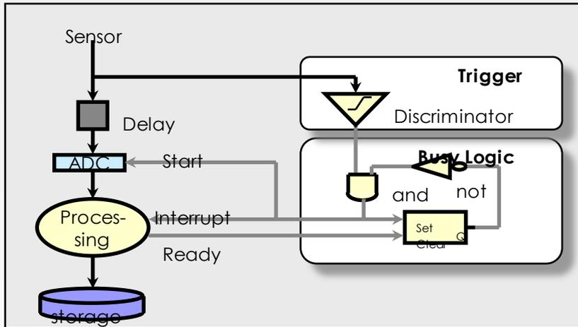
The system is *busy* during the ADC conversion time + processing time until the data is written to the storage
