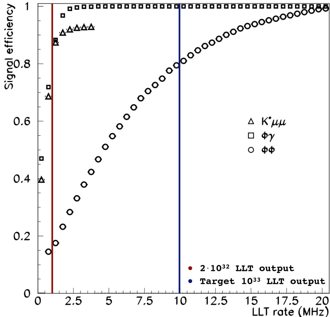
The 1 MHz detector readout is the bottleneck in the current DAQ chain
