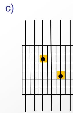
True 2D readout. Signals from wires are induced on readout plane just behind wires.
