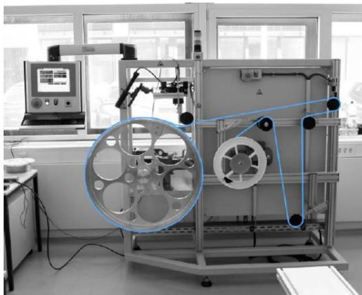
Machine for fibre mat winding
