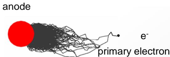
Not shown here, but important: the gas ions drifting away from the wire, produce the main part of the signal.
