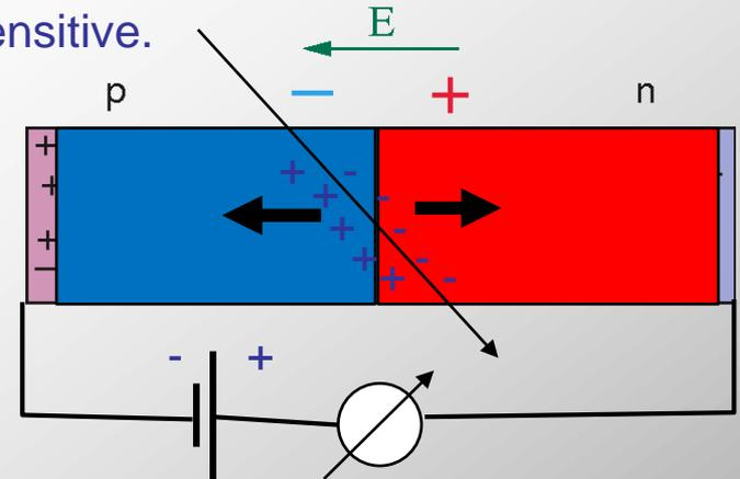
In the real world, Si-sensors are not produced by joining p and n doped material, but by implanting acceptors in a n-doped bulk (or donors in a p-doped bulk)
