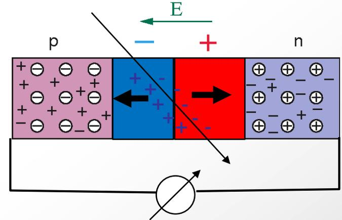
5. An external (reverse bias) voltage depletes the whole volume and makes it sensitive.
