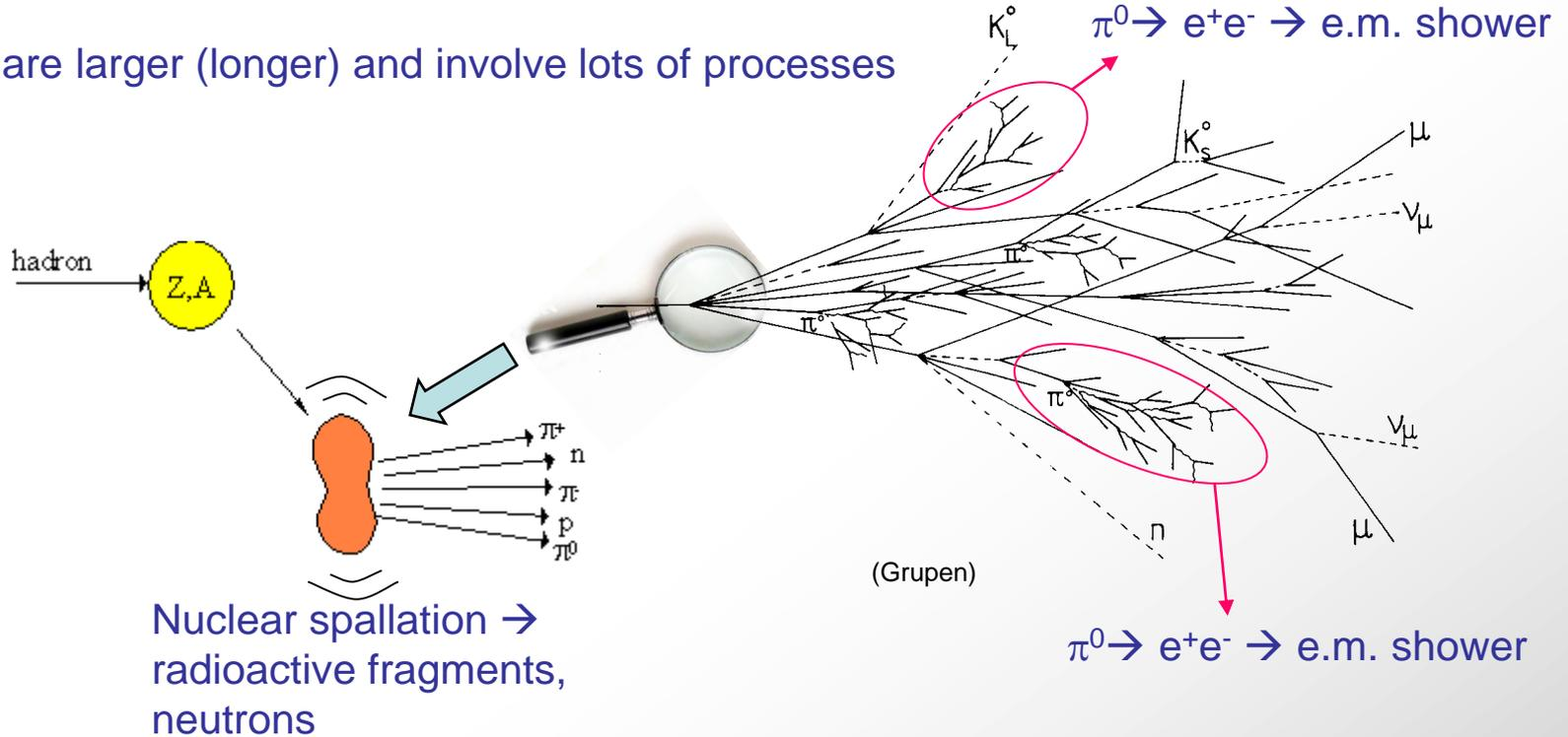
Hadronic calorimeters are larger (thicker) than electromagnetic ones. They measure the energy of neutrons and of hadronic jets (groups of close-by hadrons).
