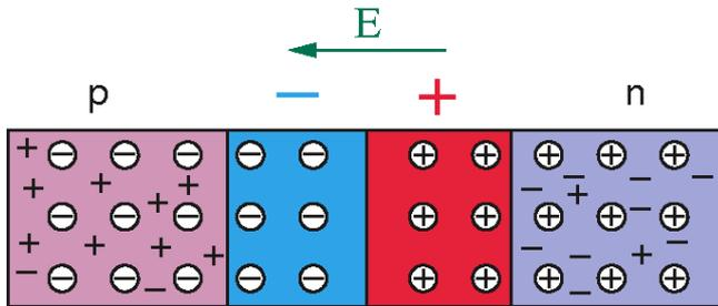
3. In the interface region holes and electrons will neutralise each other and create a depleted zone without any free charge carriers.
