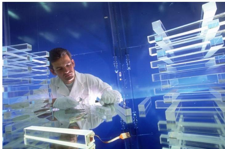
~75000  $\text{PbWO}_4$  crystals in the CMS electromagnetic calorimeter
