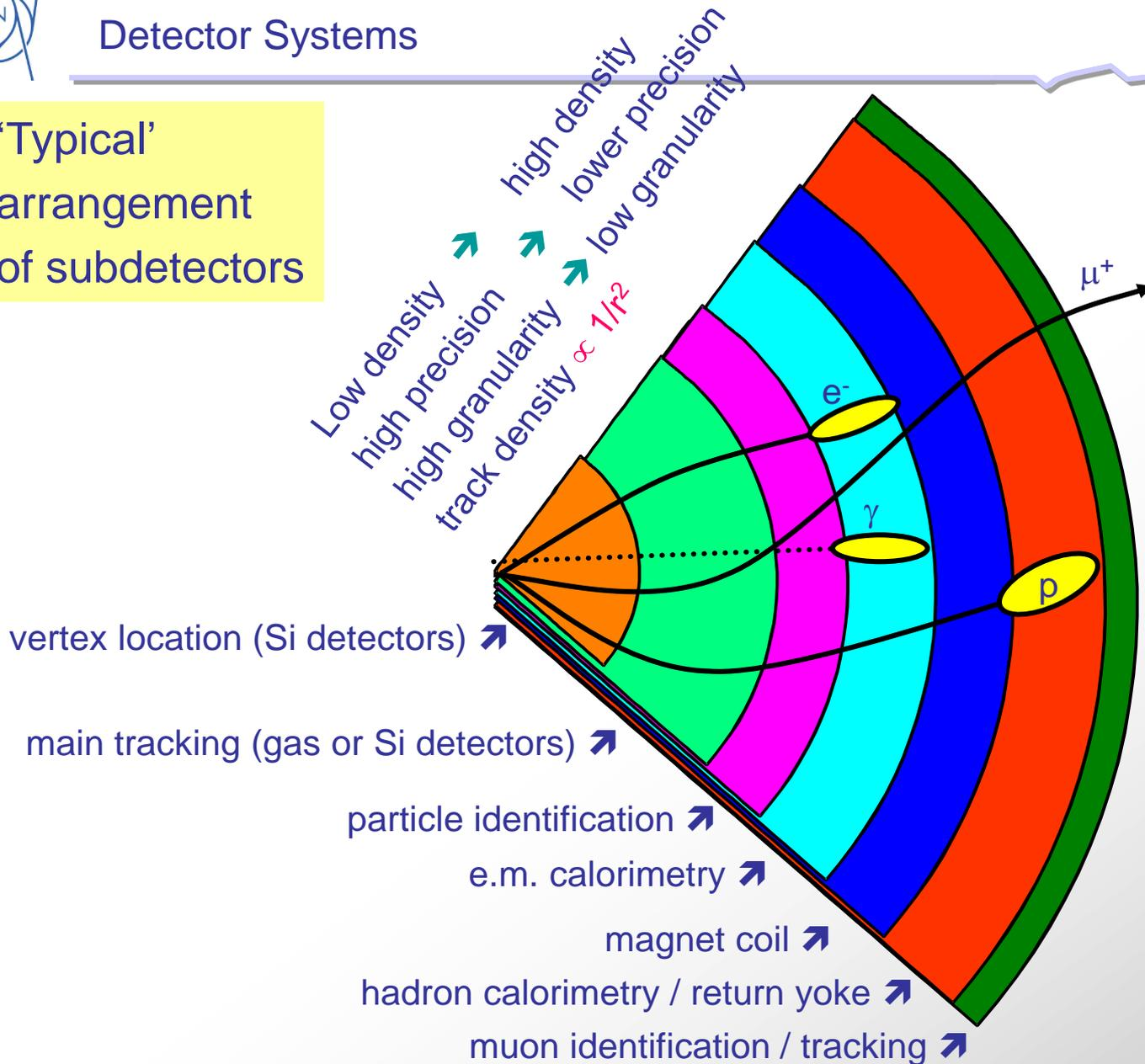
ATLAS and CMS require high precision tracking also for high energetic muons → large muon systems with high spatial resolution behind calorimeters.
