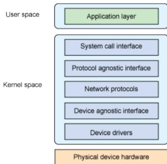
Figure: The Linux Network stack (from [9])
