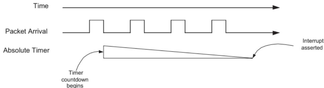
Figure: Absolute rx timer to reduce IRQs from ref. [10]
