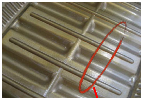
RF foil of both halves are almost touching
