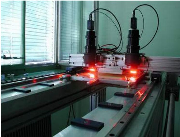
**Wire pitch and tension measurement
