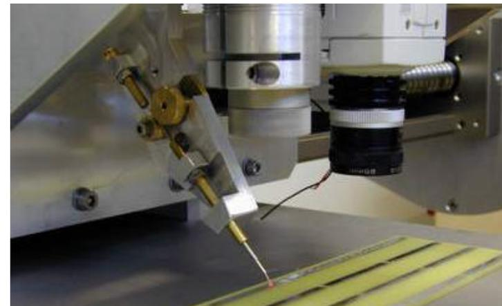
**Laser wire soldering prototype built at LNF**
