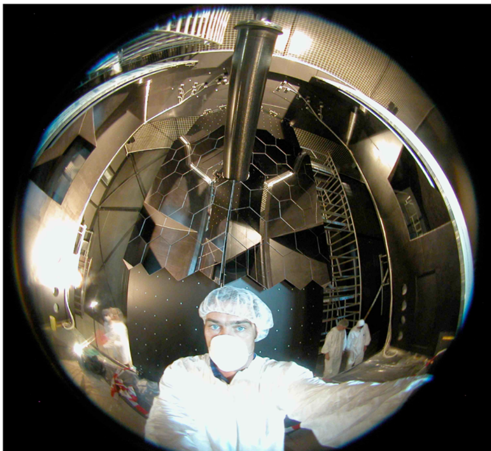
Spherical mirror alignment to 50\mu\text{rad} (spherical plus planar to 150\mu\text{rad} )
