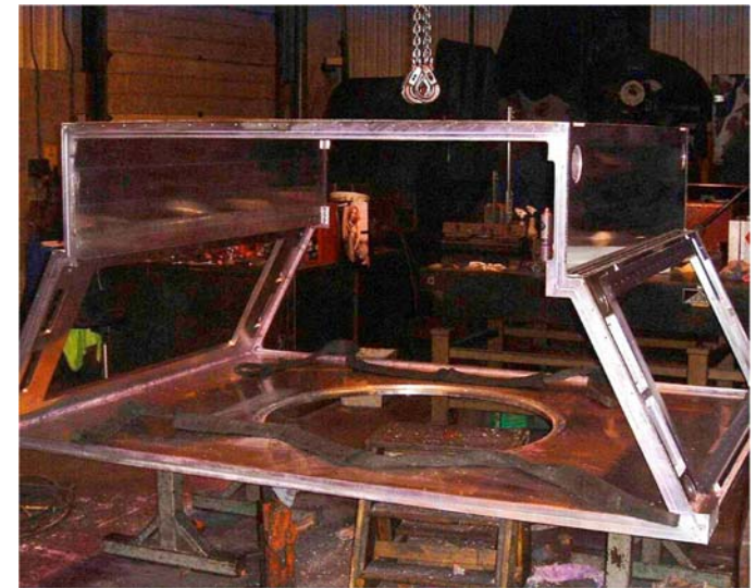
HPD shielding box aligned and fixed in the final position
