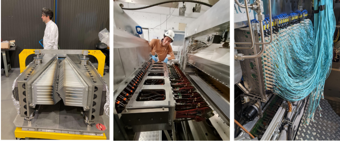
Figure 6: Left: The new boxes fixed to the trolley used to insert them in the vacuum tank. Centre: the A-side VELO half being re-inserted in the A-side box. Right: the control and data acquisition fibres reconnected to the opto-electronic boards.
