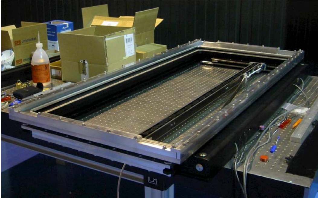
Photon funnel with B field distortion monitoring system mounted
