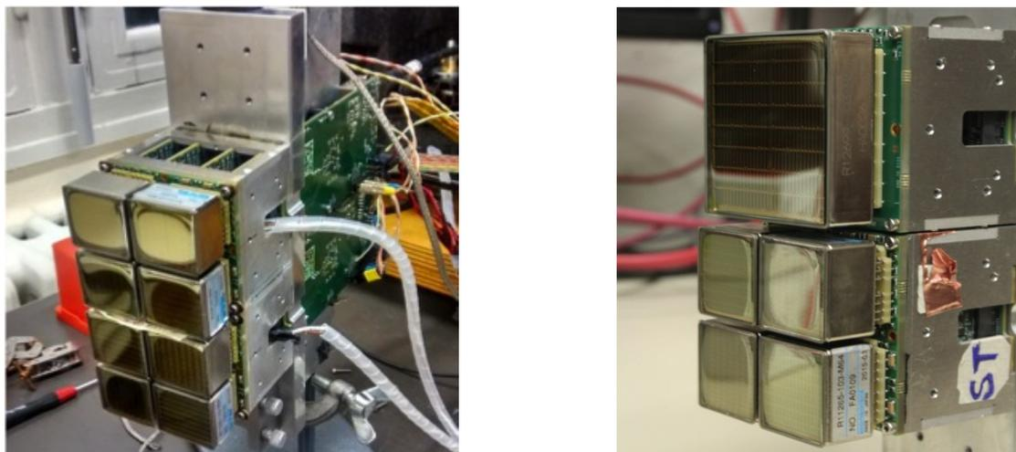
Figure 5: Left: Prototype of the photo-detector plane of the upgraded RICH used in recent beam tests. Right: prototype where both the  $3 \times 3 \text{ cm}^2$  and  $6 \times 6 \text{ cm}^2$  are mounted. The large MaPMTs are used in the outer region of RICH2.
