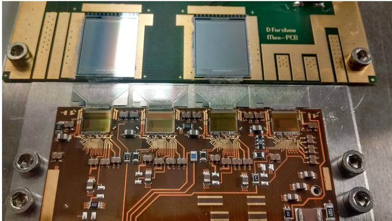
Figure 2: Hamamatsu miniature UT detectors wire-bonded to Beetle ASICs mounted on hybrid circuits to be used in May test beams. The hybridisation work has been done in the bonding laboratory commissioned for instrumented stave assembly.
