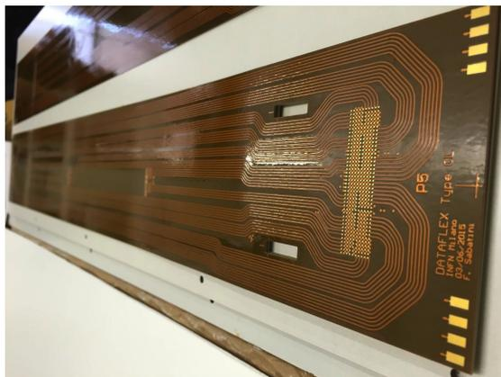
Figure 3: Prototype UT flex cable.
