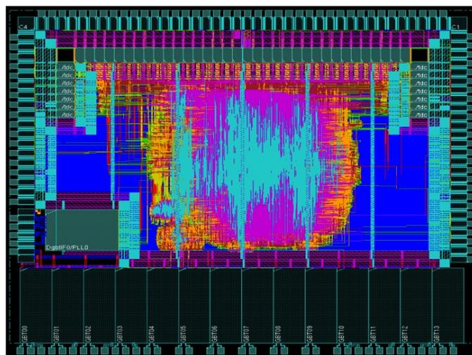
Figure 7: Layout of the muon system nSYNC chip.
