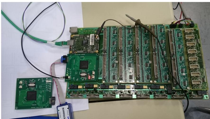
Figure 6: The new calorimeter HV control mezzanine board equipped with its radiation tolerant FPGA, plugged onto the HV motherboard.
