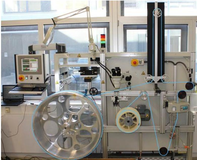
Figure 4: Winding-machine for scintillating fibre mats.
