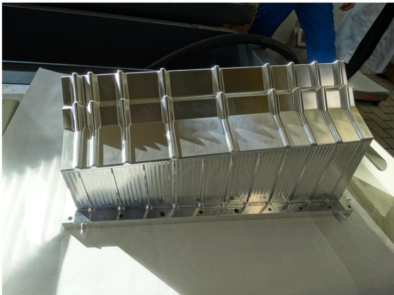
Figure 1: Half-size prototype of the VELO RF foil box.
