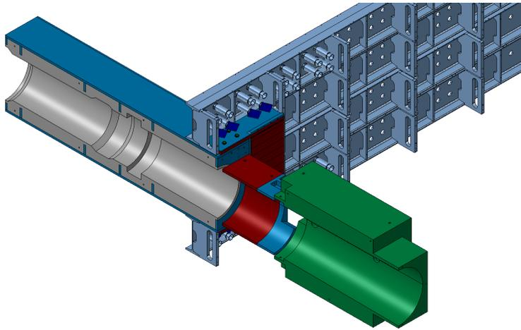
Figure 9: Design of the additional shielding in front of M2, split into three main components: the new HCAL beam plug (grey), the additional shielding behind HCAL (red), and the new M2 beam plug (green).
