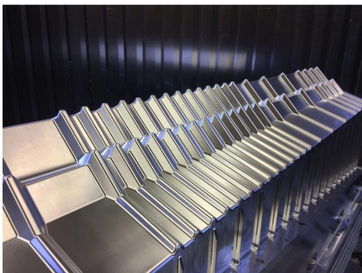
Figure 2: Full sized RF-foil prototype after machining
