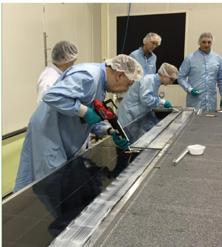
Figure 5: Assembly of a SciFi module.
