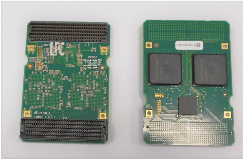
Figure 6: Revised version (v2) of the cluster board.
