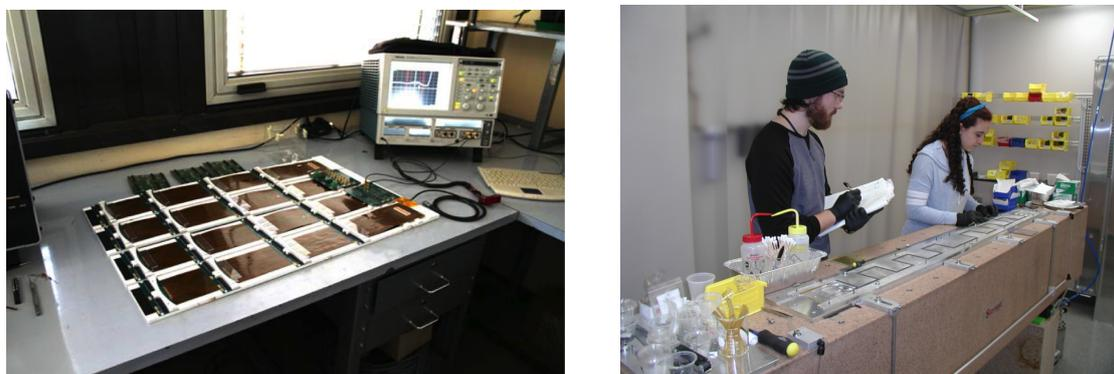
Figure 3: Left: time-domain reflectometry tests of flex cables. Right: assembly of UT staves
