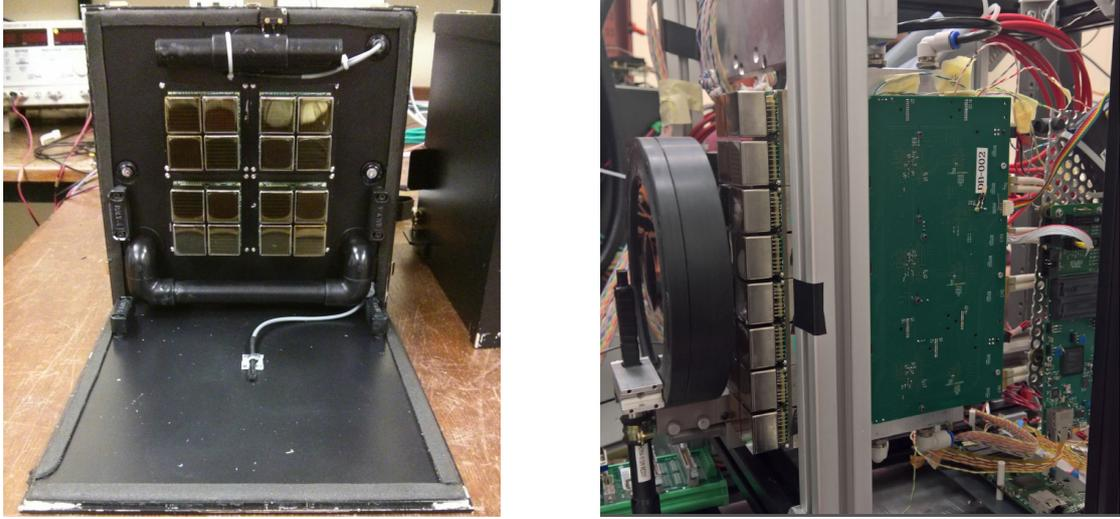
Figure 7: Left: setup for QA tests of MaPMT. Right: RICH readout demonstrator used for beam tests and read out and DAQ development.
