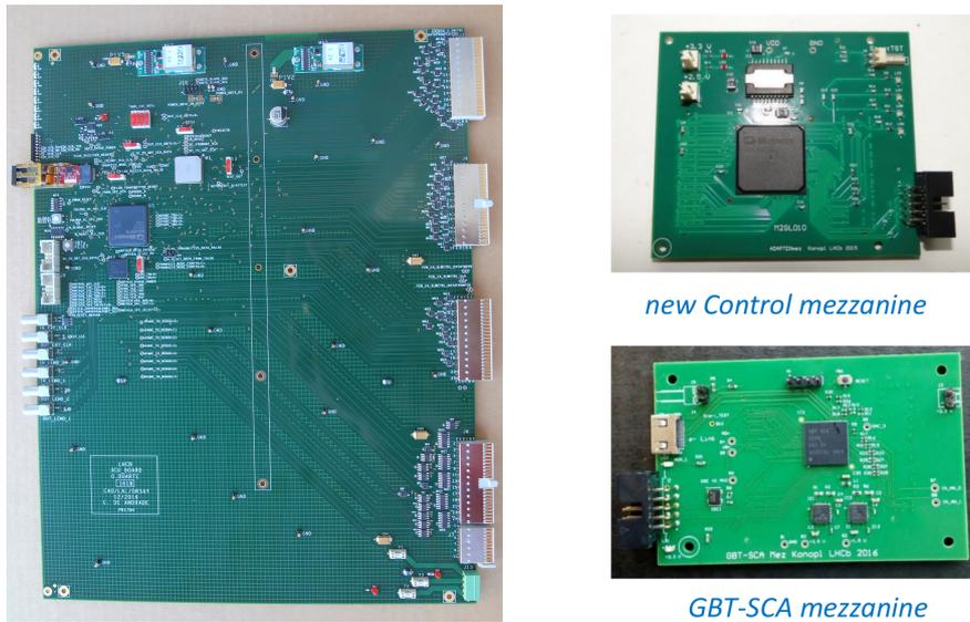
Figure 8: Left: the latest prototype of the calorimeter control board under test. Right: the two prototypes of the mezzanines designed for the high voltage, calibration and monitoring system.
