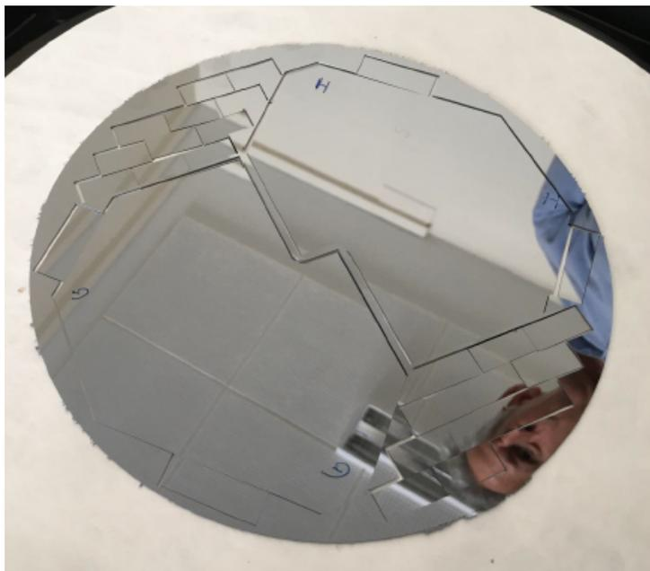
Figure 1: First test of plasma-diced microchannel wafer
