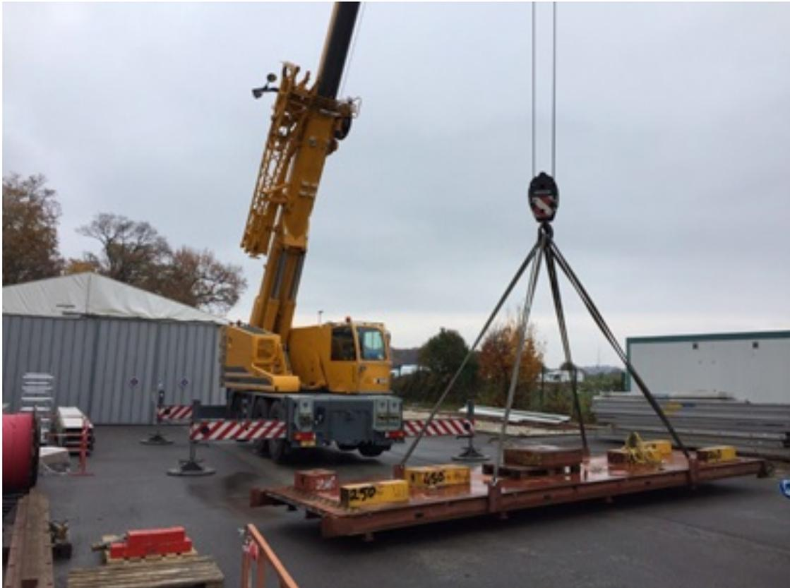
Figure 4: Load tests of the storage cradle for the lead converter.
