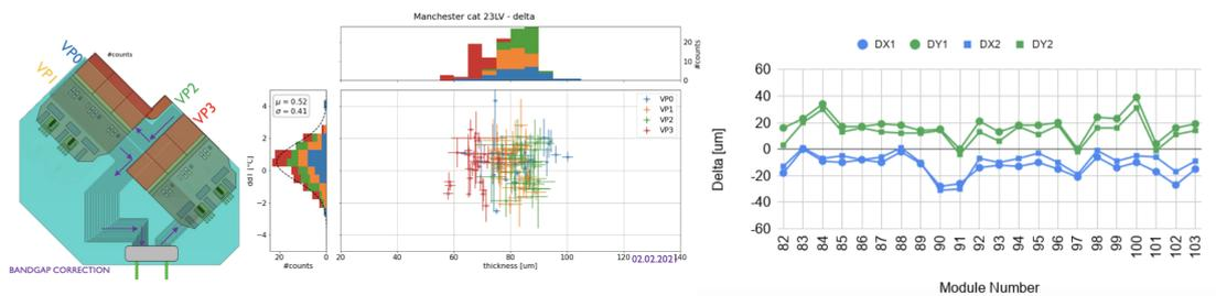
Figure 2: Quality control steps on fully assembled modules. On the left, thermal stability pre and post thermal cycling. On the right, consistency of tile positioning.
