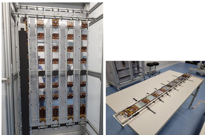
Figure 6: Instrumented staves received at CERN (left) seen in their storage cabinet in UT clean room, (right) stave 13 on the inspection station in the UT clean room, after being checked with a microscope
