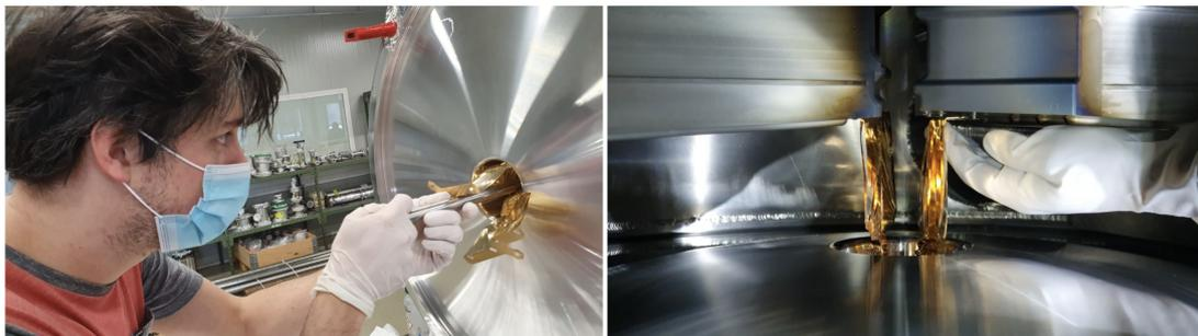
Figure 4: Photographs from the wakefield installation process. Left: Installation of the WF suppressor into the exit window Right: Final connection of the WF suppressor to the VELO RF foil
