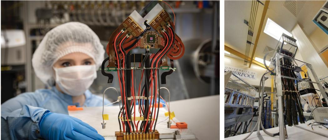
Figure 3: Photographs from the assembly process. Left: Pilot (mechanical) module being prepared for test installation on the base Right: Photograph of fully dressed vacuum feedthrough flange prior to installation
