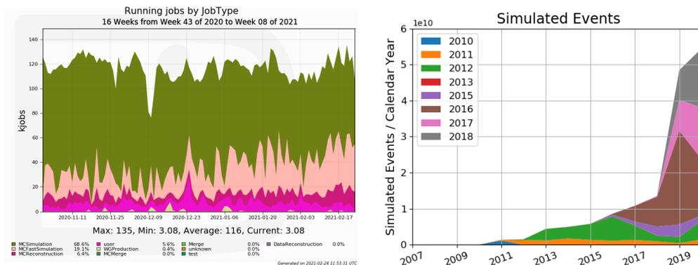
Figure 1: Left: The number of running jobs on the online-farm during the past months: the light-pink area indicates Monte Carlo jobs using a fast simulation technique, the green area Monte Carlo jobs using the full event simulation. Right: The evolution of the number of events simulated by LHCb over time. The growing usage of fast simulation techniques allows a larger number of events to be produced with similar computing resources.
