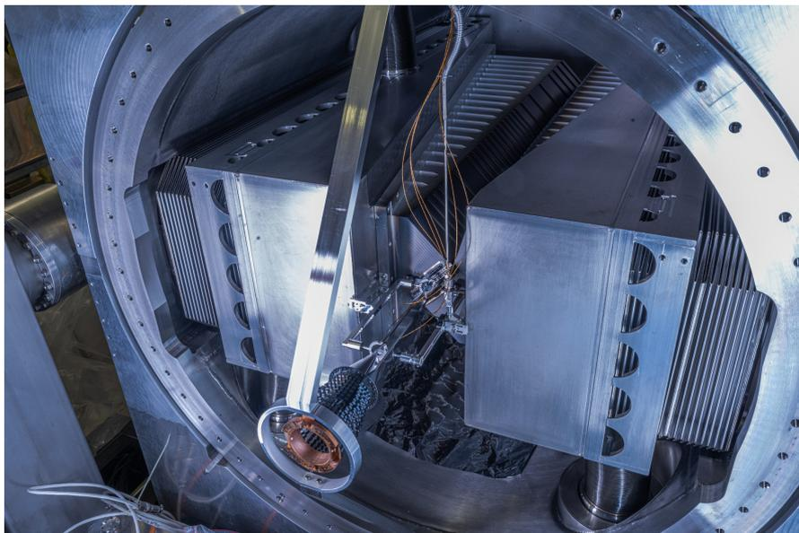
Figure 11: The installed SMOG2 storage cell with wake field suppressor, attached to the VELO RF box in the VELO vacuum vessel at IP8.
