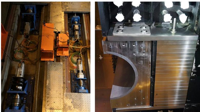
Figure 10: Left : picture of the motors to move the A and C sides of the calorimeters of LHCb. Right : the new tungsten muon filter installed in place of the hadronic calorimeter innermost cells.
