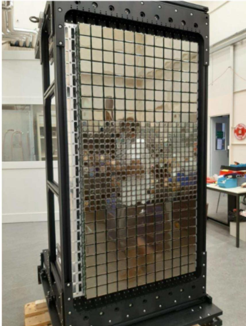
Figure 8: Complete photodetector array ready to be installed in RICH2. The two RICHes features four arrays. One of those for RICH2 has been installed after having been assembled and commissioned at CERN. The use of both 1" and 2" MaPMTs in the RICH2 design is visible.
