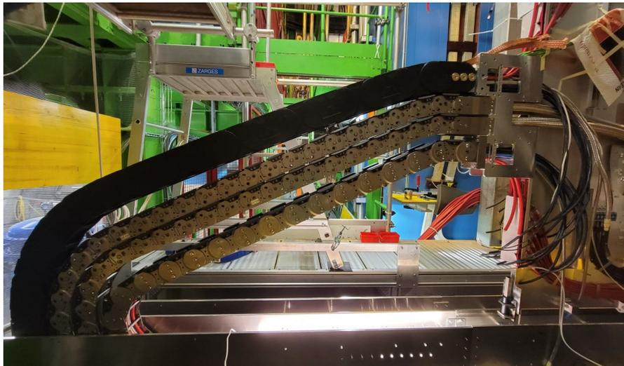
Figure 7: Test installation of the four cable chains of a single C-frame. The cable chains have been filled with cables.
