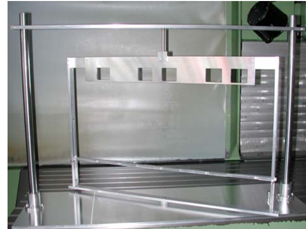
Mounting of the ladders to the cooling rod
