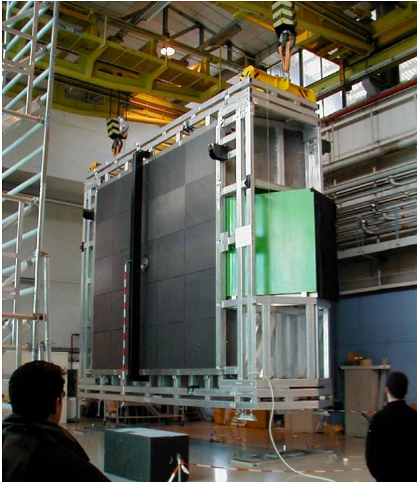
RICH2 lifting test (28t) ready for the transport
