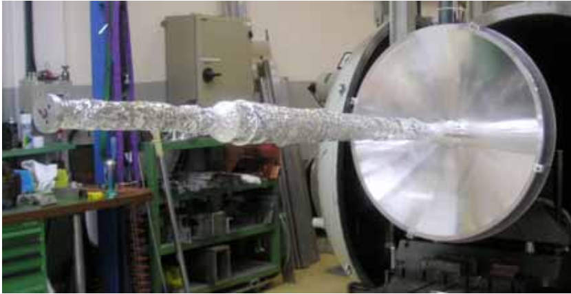
Al exit window of the VELO tank + UX85/1 Be beam pipe section
