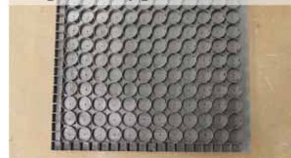
backside of the RICH-1 prototype mirror
