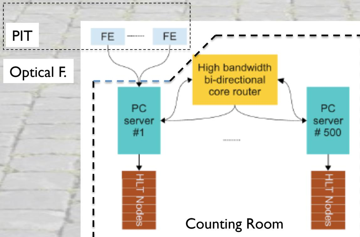
The new architecture allows a full bandwidth for data (40 MHz from “downstairs” to “upstairs”), and an efficient and lower cost event builder
