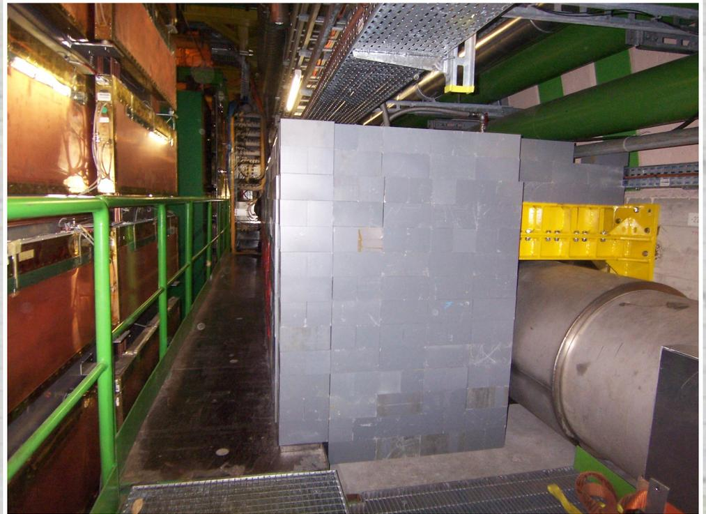
Additional shielding behind the Muon stations to reduce background in M5
