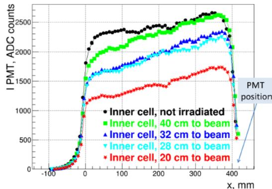
Measurements of response for module irradiated in tunnel
