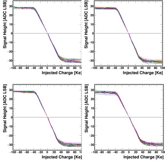
Figure 3: Study of the dynamic range of the four SALT chips integrated in a flex-hybrid prototype included in the slice test shown in Fig. 2.
