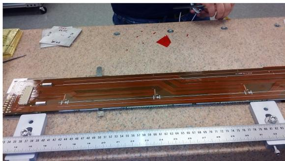
Figure 4: A flex cable glued onto a prototype stave.
