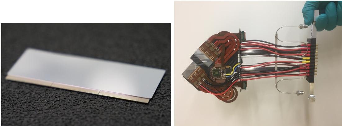
Figure 1: Left: an assembled tile. Right: an assembled prototype VELO module.
