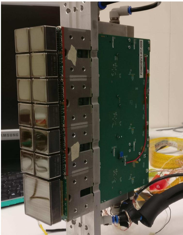
Figure 8: Photograph of a complete Photon Detector Module.
