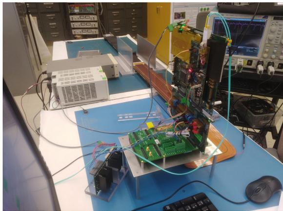
Figure 2: Electronics configuration for the first UT slice test: a hybrid is mounted on the farthest location from the peripheral electronics and communicates with it via a final-design prototype flex cable.
