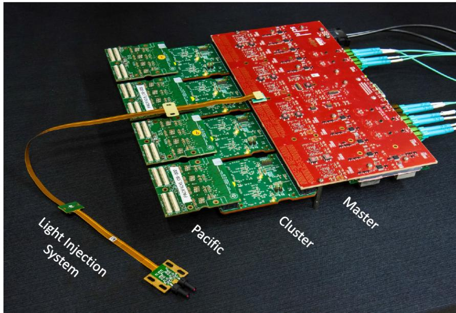
Figure 6: Photograph of the electronics readout chain.
