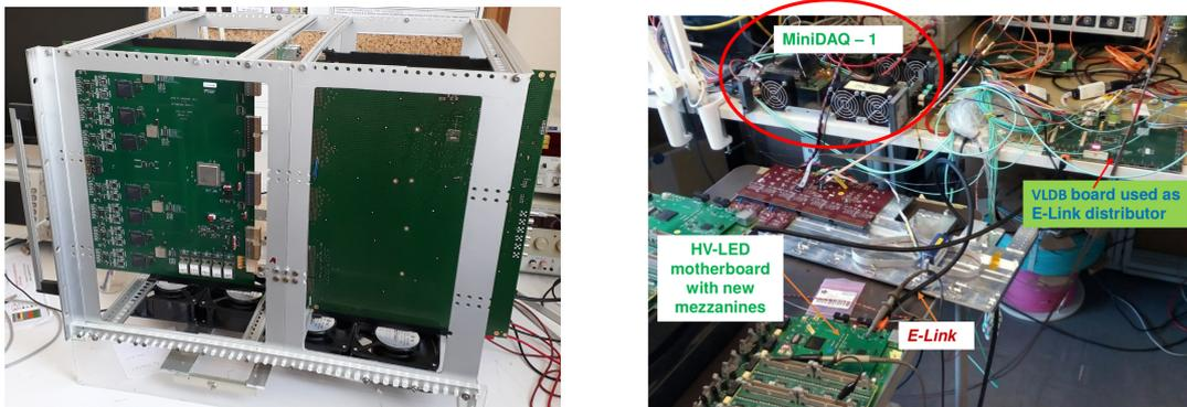
Figure 9: Left, picture of the common tests performed with the FEB and the control board in a specific crate, giving an easy access to the system. Right, picture of the HV/Calibration/Monitoring systems under tests with the MiniDAQ at CERN.
