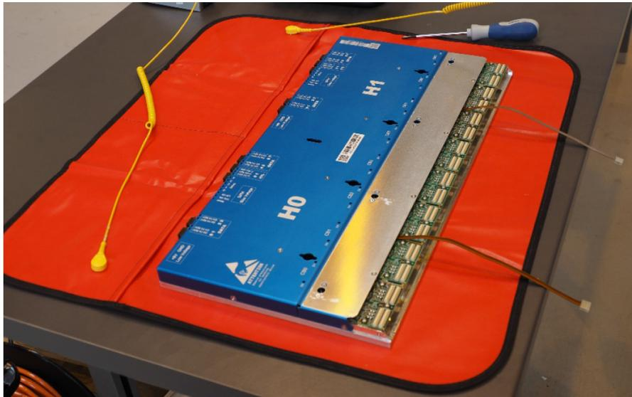
Figure 8: Photograph of a finished readout box (ROB) containing 8 PACIFIC carrier boards, 8 cluster boards and 2 master boards
