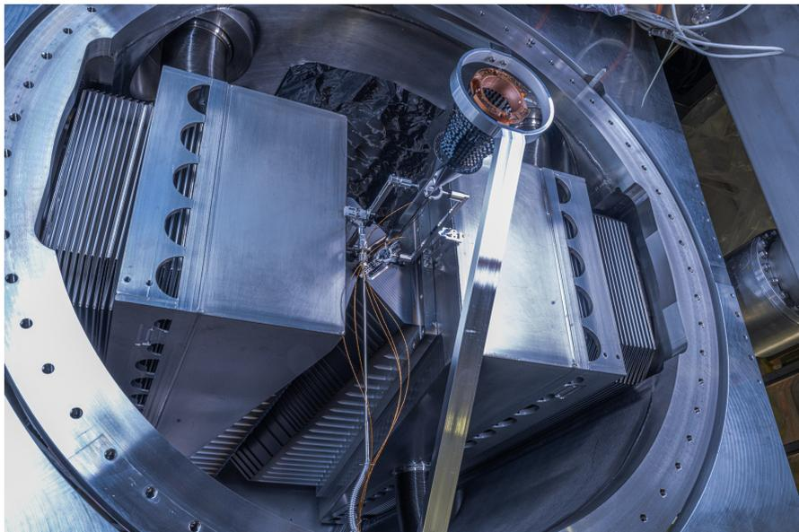
Figure 13: The installed SMOG2 storage cell with wake field suppressor, attached to the VELO RF box in the VELO vacuum vessel at IP8.
