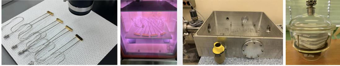
Figure 2: Some of the microchannel procedures developed to deal with Covid-19 working practice. From left to right: optical inspection of connectors, plasma cleaning of multiple connectors, new vacuum tank for storage of multiple connectors before metallisation, new vacuum storage of multiple solder foils.
