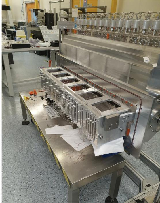
Figure 4: VELO C side base and hood, fully installed with cooling runs and tertiary vacuum system
