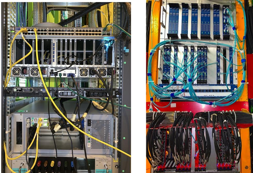
Figure 12: The Muon commissioning rack (left) and the Q1M45 Muon rack (right), fully equipped with new readout and control electronics
