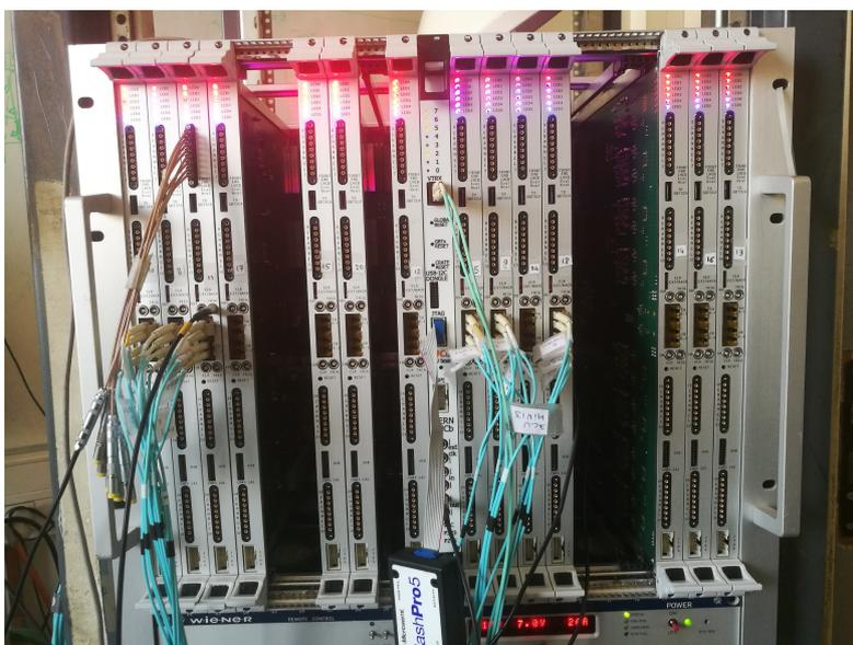
Figure 11: Test bench of the calorimeter equipped with pre-production FEBs.
