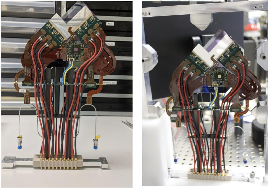
Figure 3: The first post lockdown modules to be produced: M82 (Manchester) on the left; M13 (Nikhef) on the right
